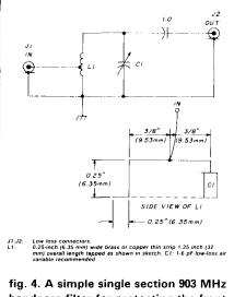
bandpass filter for protecting the front end of a receiver. Bandwidth is approximately 100 MHz and insertion loss is 0.5 dB maximum.
